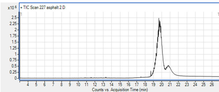
Figure 2. TIC of 4 mg of asphalt binder desorbed at a temperature of 300 °C.
